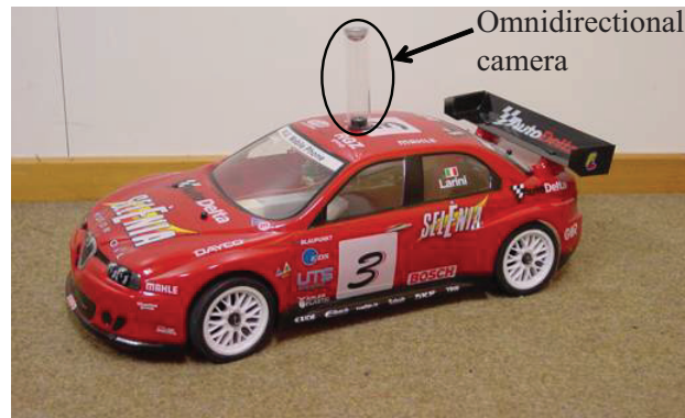
Figure 2.5: A 1/10 scale model car equipped with omnidirectional camera.
