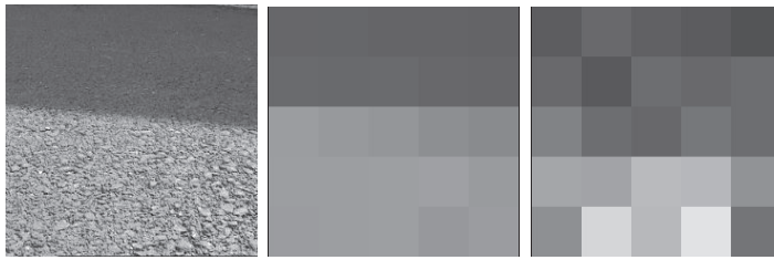
Figure 5.2: Left: Snapshot from the robot camera. Center: Pixel average. Right: Pixel sample.
