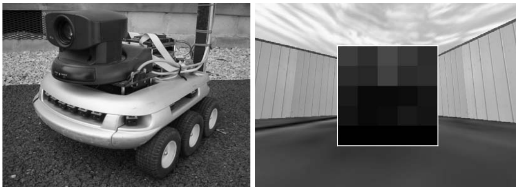
Figure 3.1: Left: The original six-wheeled robot Koala equipped with a pan/tilt camera. Right: The robot's perspective in a simulated environment. The robot can access the world with 5 by 5 retina at the center of the image.
